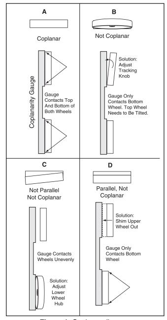
Figure 1. Coplanar diagram.
